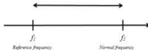
Figure 1: A typical situation in frequency metrology, a well-known reference frequency and an unknown frequency tens or hundreds of THz apart.
